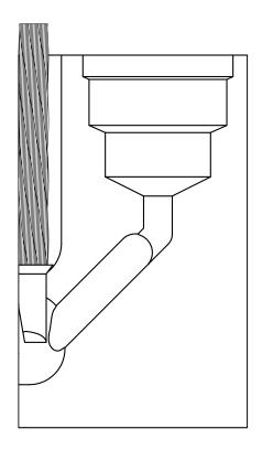
1. Push formed terminal (bond-end) into the mold until it stops
