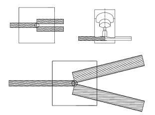
Butt cables under center of tap hole, as shown.
