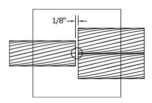
When all conductors are larger than 750 MCM, gap cables 1/8" under center of tap hole.
