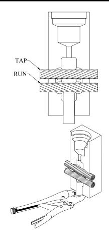
Place cables into mold. Bottom run cable must sit on top of the ground rod. Use locking pliers or a clamp on the rod below the mold to prevent it from slipping when the mold is fired.
