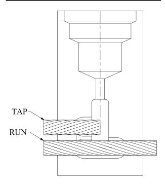
Place end of tap cable under center of tap hole. Do not cut run cable or try to splice cables in this mold.
